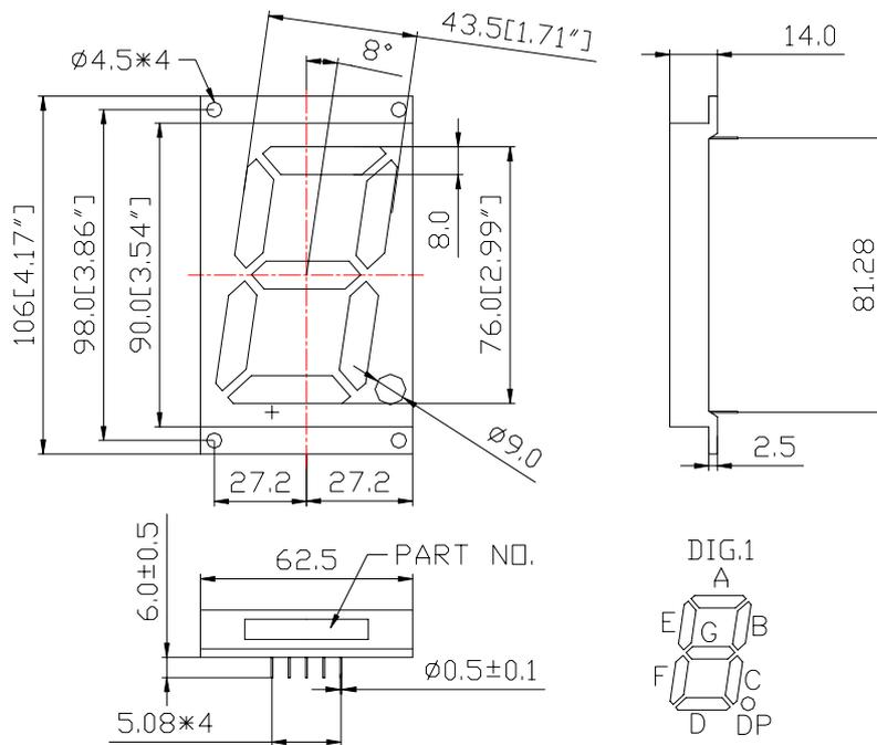
NOTES: All dimensions are in millimeters (inches) tolerance are  $\pm 0.25\text{mm}(0.010)$  unless otherwise noted.
