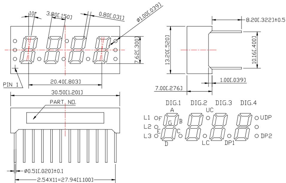
NOTES: All dimensions are in millimeters (inches) tolerance are  $\pm 0.25$ mm(0.010) unless otherwise noted.
